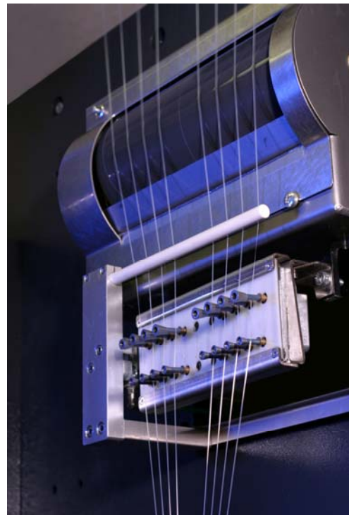
FibreTOS Oil Sensors on Barmag FDY Machine
