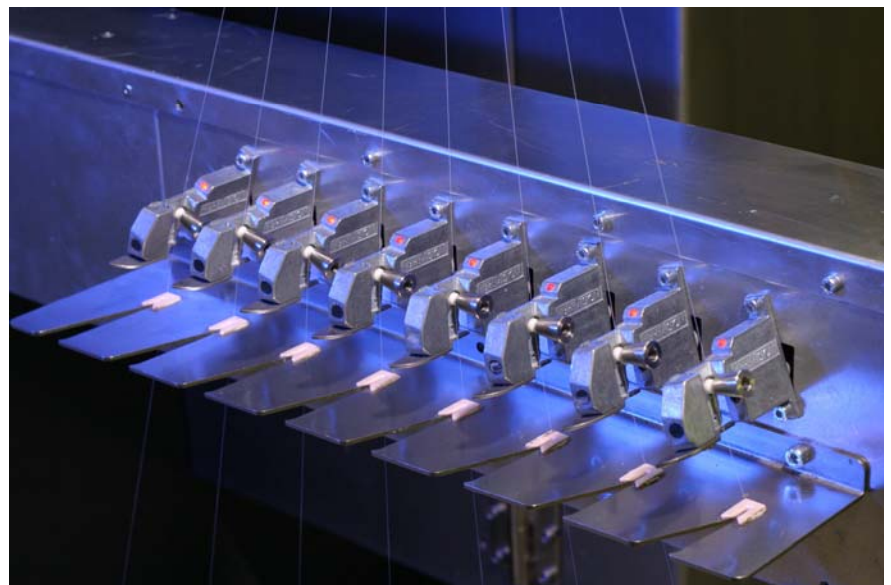
FibreTOS Optical Sensors Fitted to Barmag FDY Machine
